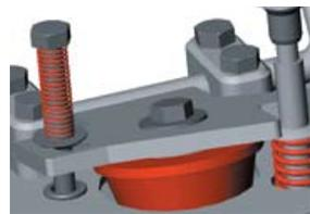
**Spring-balanced valve control system.**
