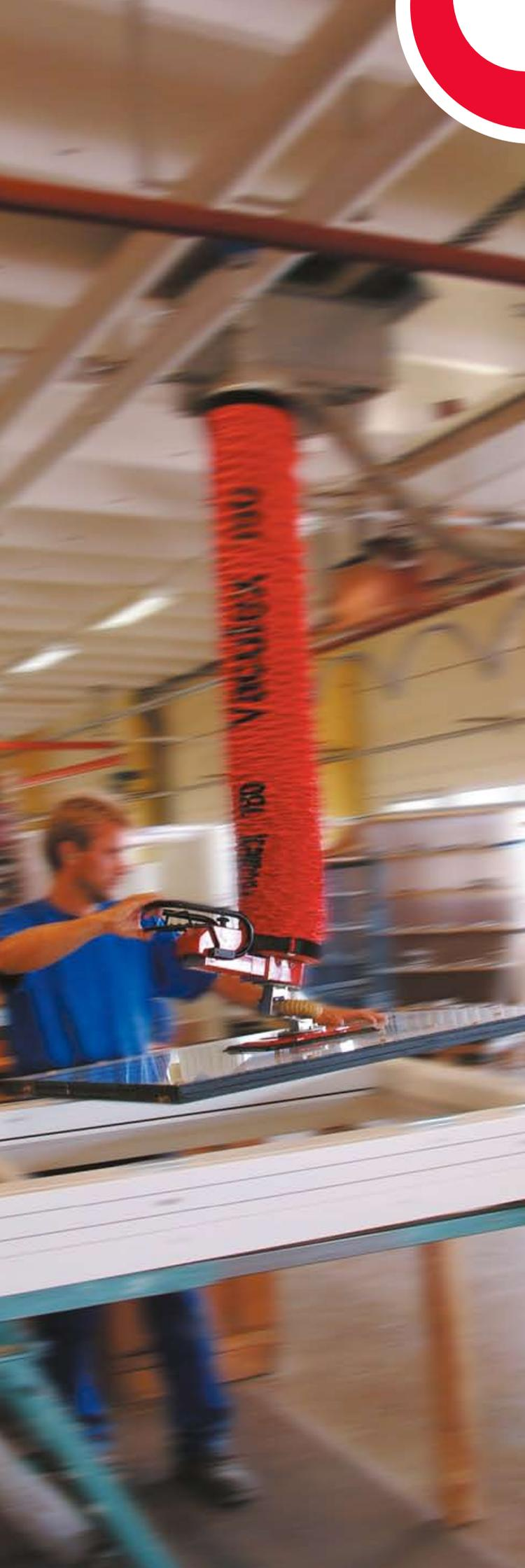
A worker in a blue shirt is operating a red vacuum tube lifter in a factory setting. The lifter is a vertical red tube with a suction foot at the bottom, used for lifting objects. The worker is holding a control unit connected to the lifter. The background shows a factory floor with various equipment and structures.
